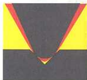
COMPARISON OF CONVENTIONAL ELLIPTICAL STYLUS (BLACK) TO SHIBATA-TYPE STYLUS (RED). SHIBATA-TYPE TRACES MORE OF THE GROOVE INFORMATION AND PLACES LESS TENSION UPON THE DISC SURFACE.
